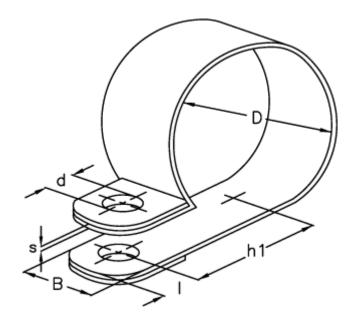
$\begin{array}{ll} d & = 10.5 \\ \text{Diameter D} = 70 \\ \text{h1} & = 49.5 \\ \text{I} & = 10.0 \\ \text{s} & = 1.2 \\ \text{Width B} & = 25 \\ \end{array}$
